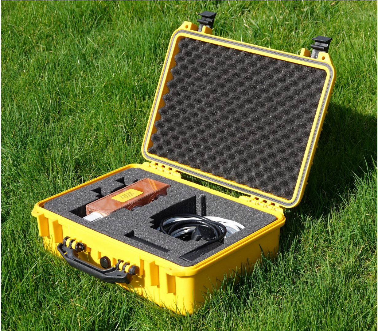
Figure 1. PPMG4A Proton Precession Magnetometer
